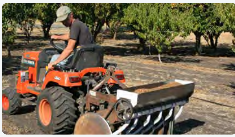
A home-built no-till seed drill, shared under a Creative Commons Attribution 4.0 International License by Sunny Slope Orchard (2013).
